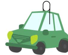
3. Cut and attach two strips of Maker Tape to the vehicle that go from each of the LED legs to the bumper of the vehicle. Make sure the two strips of Maker Tape do not touch each other.
